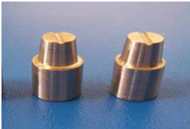
Fig(1) : Stainless steelworkingdies
