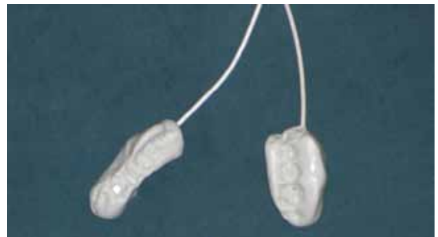
5. Load cell and metal piece in silicone putty
